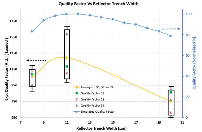
Fig. 6: Preliminary experimental and simulation results for the 5 th -order TPoS resonator with different trench widths.
